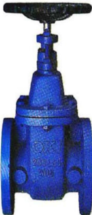
Non-Rising Stem, Inside Screw, Bolted Bonnet, Solid Wedge Disc, Flange to B16.10
